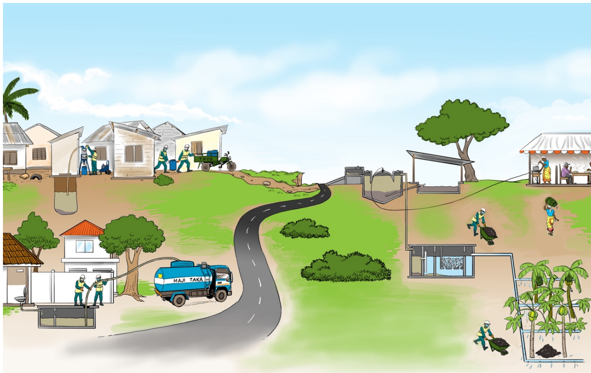
Figure 1: The FSM “service chain” for the specific context of Dar es Salaam
