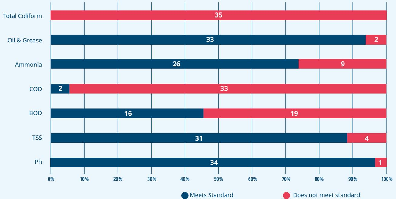
**Fig. 35:** CBS systems in Sleman – effluent parameters complying with regulations [46]
