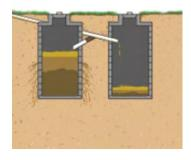
**Double leach-pit:** Two alternating partially lined (sealed on the bottom) pits, where one pit is used until it becomes full. At the same time, wastewater slowly permeates into the surrounding soil, which allows the easy removal of degraded, dewatered soil.
