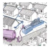
**Small or simplified sewer network connected to off-site septic solution:** Small sewerage networks are constructed using smaller diameter pipes laid at a shallower depth and a flatter gradient than conventional sewers. Typically these pipes lead to a decentralised wastewater treatment solution (DEWATS).
