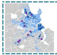
Centralised water supply network refers to a vast network of underground pipes, which connect water sources (e.g. ground of surface water) directly to the end users.
