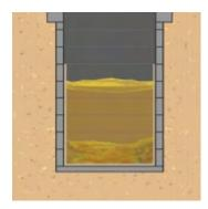
**Lined-pit:** A single or double hole lined with sand-cement rings, trapezoidal cement blocks or normal blocks, **which might also be raised off the ground in areas with high water table or flood-prone.** Lined pits are more permanent and long lasting than unlined-pits, and preventing soil from collapsing. Sludge can be easily removed and the pit re-used many times (See Page 8).
