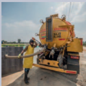
"Honeysucker" in Devanahalli, Faecal Sludge Treatment Plant
