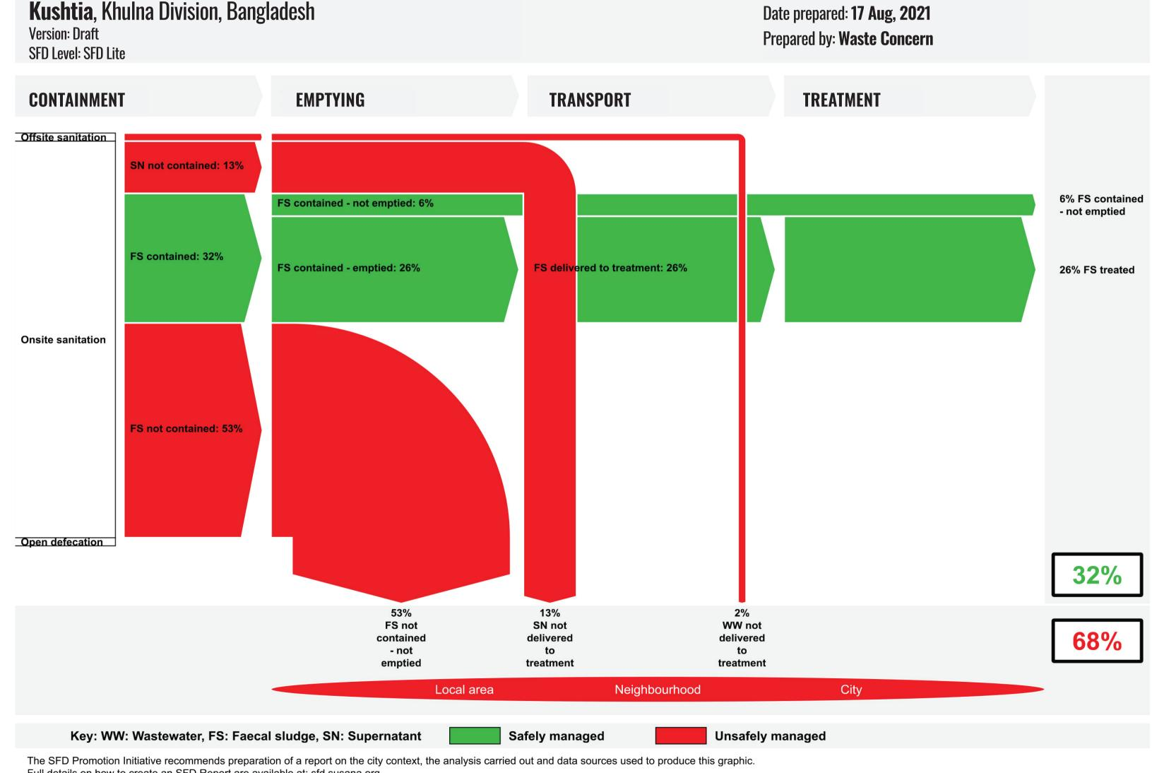
Kushtia Municipality does not have sewerage network and sewage treatment plant installed within its municipal area. Wastewater from disperse homesteads of the fringe area is drained and discharged into adjacent ditches or open drains. Wastewater and runoff from buildings, streets, parking lots, driveways, lawns and other areas collected by tertiary drains and discharged into rivers and khals.
