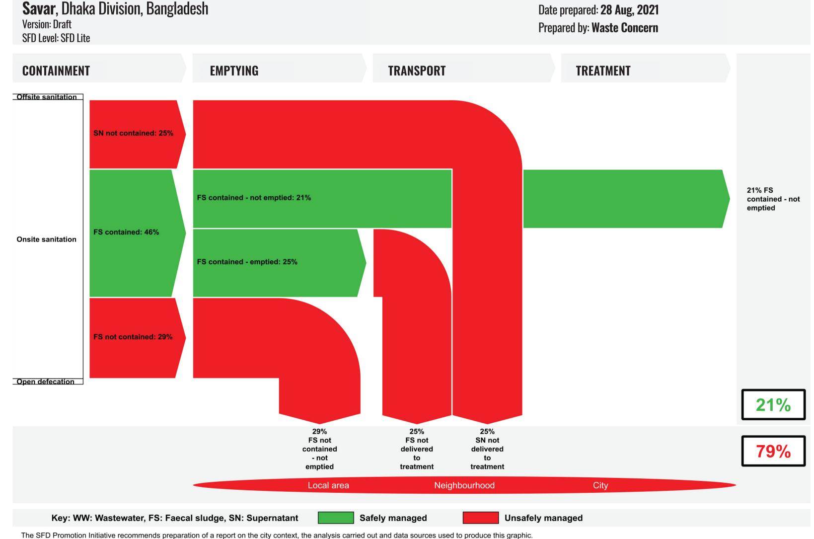
Savar Municipality does not have sewerage network and sewage treatment plant installed within its municipal area. Wastewater from disperse homesteads of the fringe area is drained and discharged into adjacent ditches or open drains. Wastewater and runoff from buildings, streets, parking lots, driveways, lawns and other areas collected by tertiary drains and discharged into rivers and khals.
