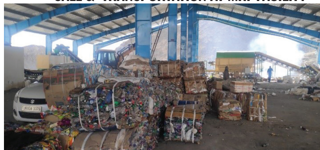
FIG 30 : BAILED RECYCLABLES PACKED FOR SALE & TRANSPORTATION AT MRF FACILITY
