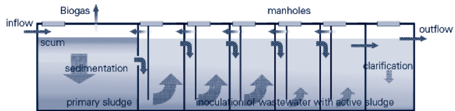
Picture 9_13: Flow principle of a baffled septic tank. Incoming wastewater is forced to pass through active-bacteria sludge in each compartment. The settler at the front prevents larger solids from entering the baffled section
