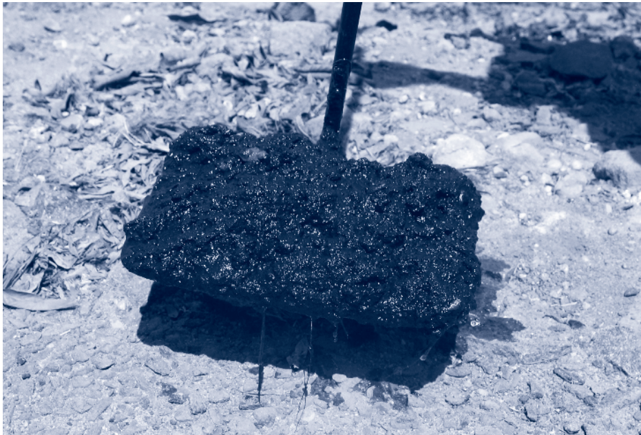
Picture 8_4: Sludge from an septic tank in India – the black colour of the sludge indicates anaerobic condition
